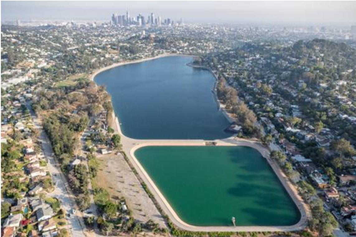
*A new aeration system will use the existing spillway between the two reservoirs and is designed to slow algae growth and reduce potential related odors from anaerobic conditions. (Photo: LADWP)*
